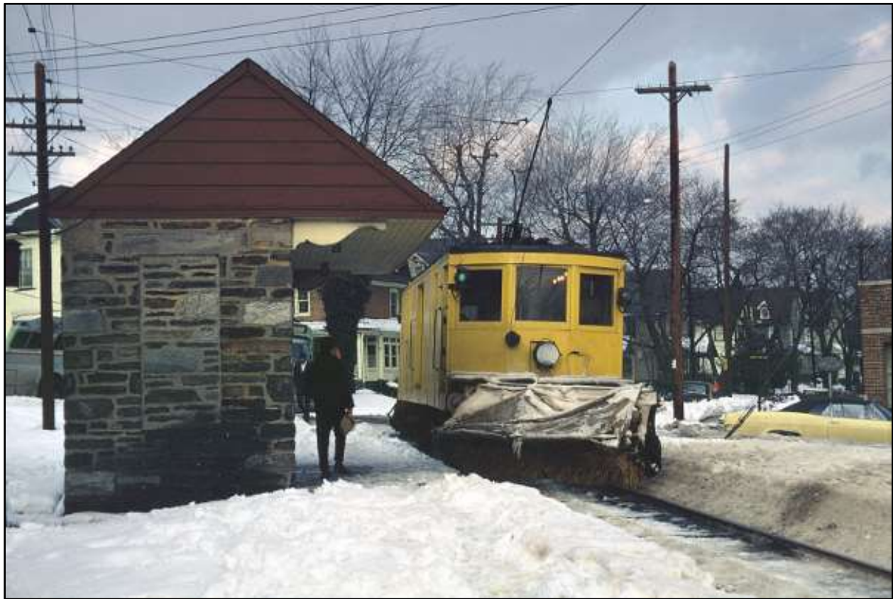
Red Arrow #4, a snow sweeper trolley with spinning horizontal brushes, pauses at County Line Road station after the blizzard of December, 1966. This location became the eastern end of the busway three months later. (photograph by Robert Coolidge; used with permission.)
