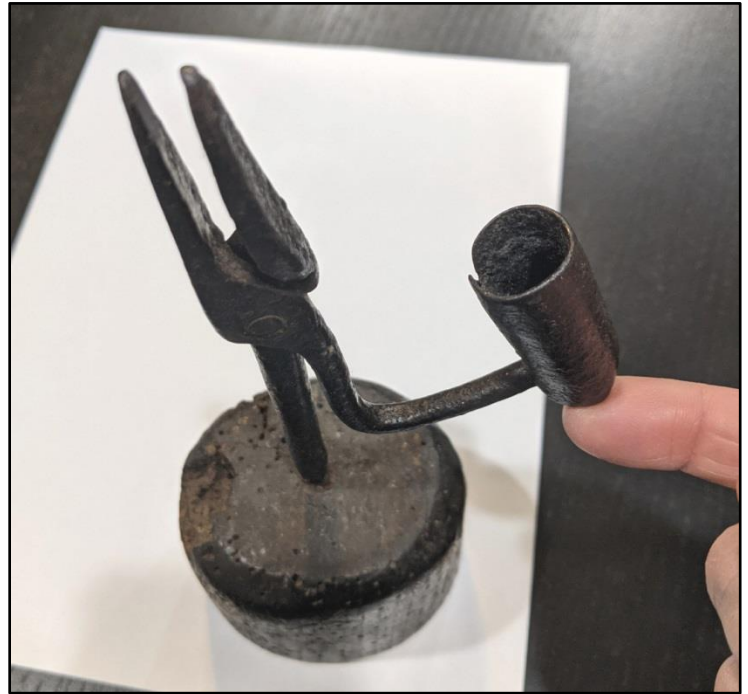
Home again: The HTHS rush light is a combination light, with a hinged rush holder and a side-mounted candle holder.
